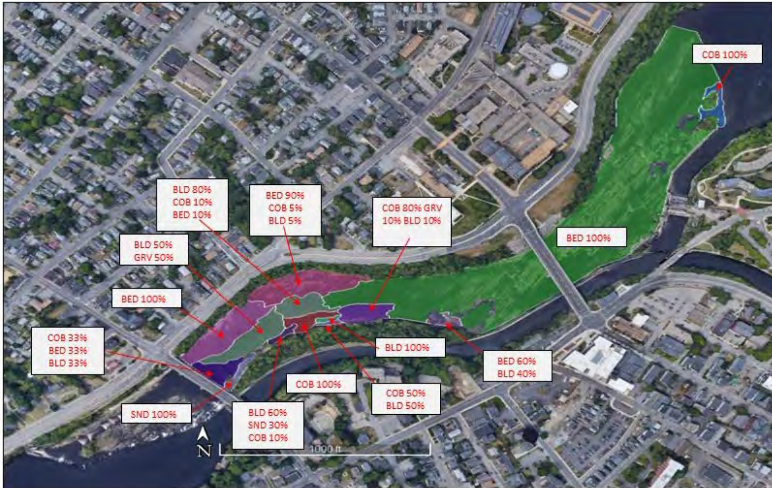
Figure 4–1. Substrate polygon map of the Bypass Reach. See Section 4.2.3 for substrate code.
