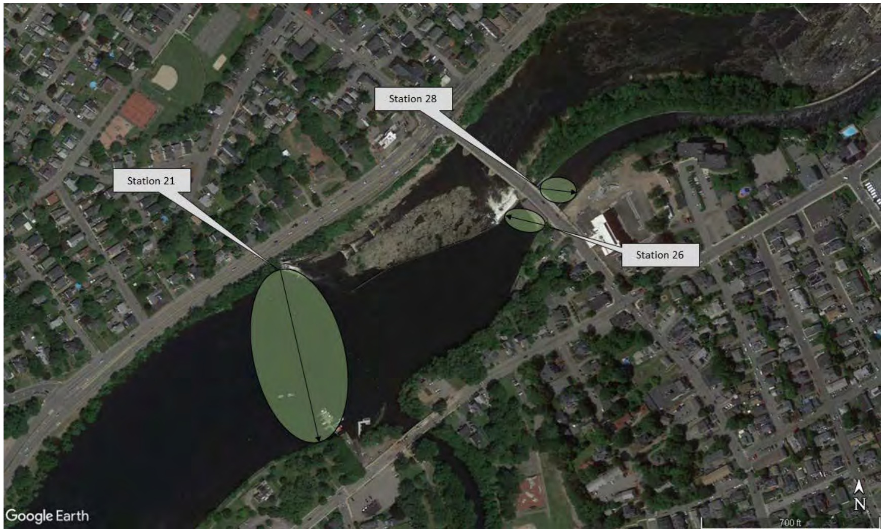
Figure 4–2. Locations and approximate detection areas for stationary radio-telemetry receivers installed upstream of Pawtucket Dam and at the Northern Gatehouse during the 2019 juvenile alosine downstream passage assessment at Lowell.
