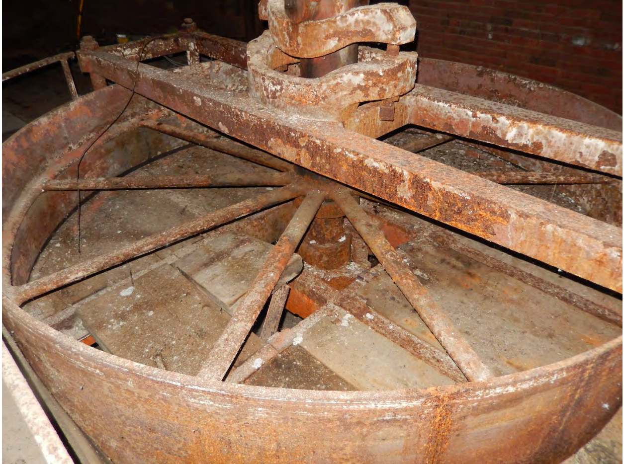
Figure 5-3. Belt drive sheave mounted atop Francis turbine.
