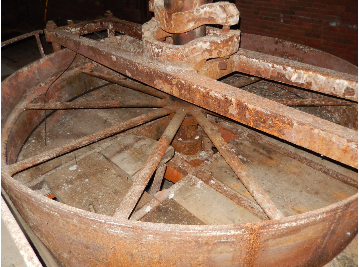
Figure 5-3. Belt drive sheave mounted atop Francis turbine.
